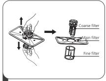
The fine filter can be pulled off the bottom of the filter assembly.
