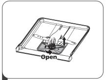
1 Hold the coarse filter and rotate it anticlockwise to unlock the filter. Lift the filter upwards and out of the dishwasher.
