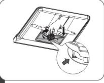
Reassemble the filters in the reverse order of the disassembly, replace the filter insert, and rotate clockwise to the close arrow.
