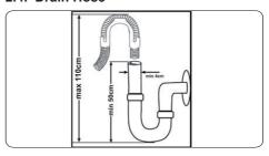
Connect the water drain hose directly to water drain hole or to the sink outlet spigot. This connection should be minimum 50 cm and maximum 110 cm from flor plane.
