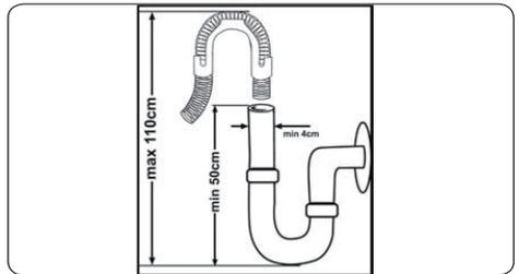
Connect the water drain hose directly to water drain hole or to the sink outlet spigot. This connection should be minimum 50 cm and maximum 110 cm from floor plane.
