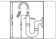
Connect the water drain hose directly to water drain hole or to the sink outlet spigot. This connection should be minimum 50 cm and maximum 110 cm from flor plane.
