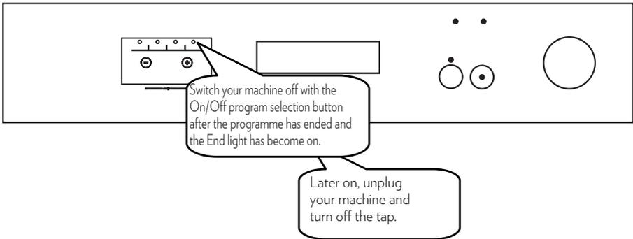
**NOTE:** In order for the drying process to be performed more quickly, you may slightly open the machine door after few minutes when the programme has ended and the End light has been lit.
